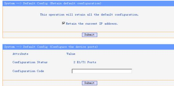
H0FL-EthMux.SA16 series device supports changing E1/T1 port number. For example, change E1/T1 port number of H0FL-EthMux.SA16 to 1. It is shown as follows:
