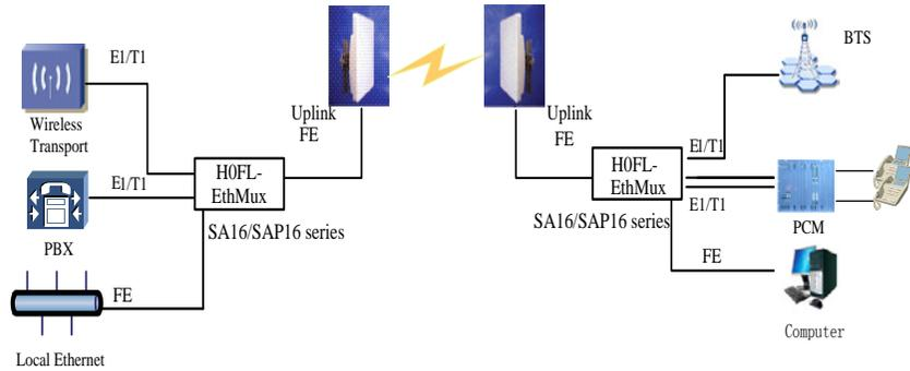
**Figure 2-3** Typical application of HOFL-EthMux.SA16/SAP16 series device in cable network
