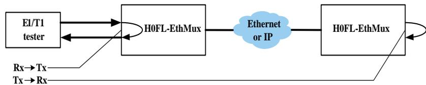
Rx→Tx can test E1/T1 connection cable, and Tx→Rx is used to test the whole circuit including H0FL-EthMux.SA16/SAP16 series devices at both ends and the Ethernet link between them.
