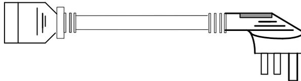
The AC power cable which meets Japanese/American standard (ZJN.BH4.855.035-E) is composed of Japanese standard two-plug connector and pins terminal, as shown in Figure 4-10.
