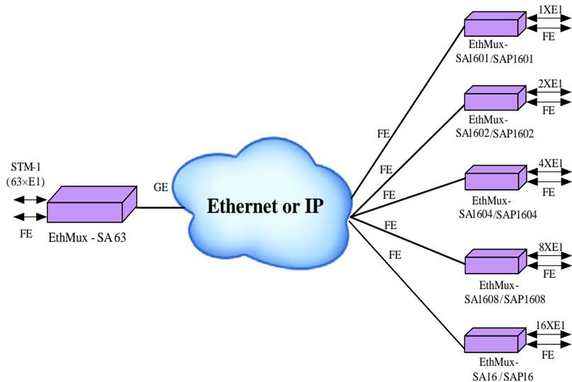
**Figure 2-2** Typical application of HOFL-EthMux.SA16/SAP16 series devices in wireless network
