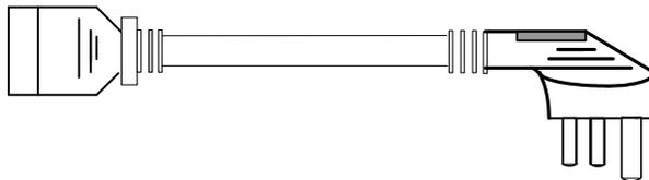
The AC power cable which meets German standard (ZJN.BH4.855.035-B) is composed of German standard French-mode two-plug connector and pins terminal, as shown in Figure 4-8.
