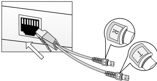
**Step 4** Aim the bayonet of BNC cable's male interface at the standoff of interface conversion cable BH4.850.122's BNC interface, then insert it into the standoff with moderate force and turn it right to the slot, as shown in Figure 5-8.
