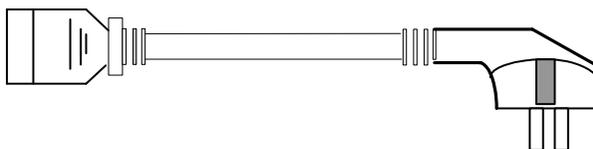
The AC power cable (ZJN.BH4.855.080-D) which meets South Africa standard is composed of South Africa standard three-plug connector and pins terminal, as shown in Figure 4-3.
