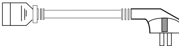
The AC power cable which meets South Africa standard (ZJN.BH4.855.035-D) is composed of South Africa standard three-plug connector and pins terminal, as shown in Figure 4-9.
