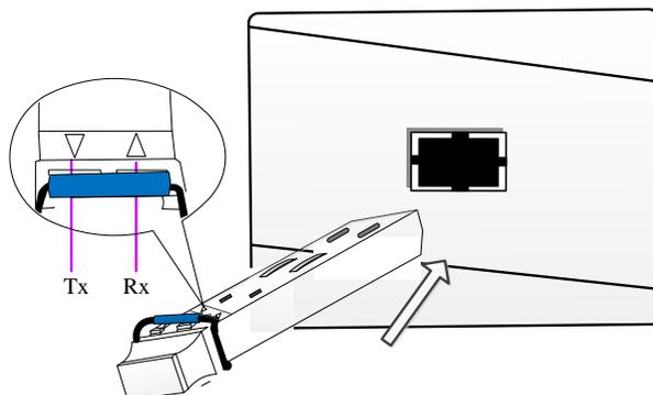
**Step 2** Respectively remove the dust caps on the optical module and the optical fiber, aim the head of the fiber at the optical module port and insert it into the port with moderate force.
