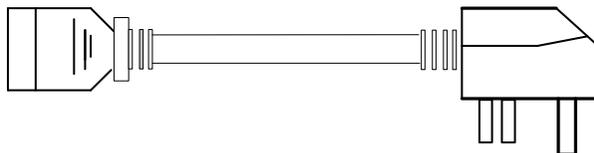
The AC power cable (ZJN.BH4.855.080-G) which meets North American standard is composed of North American standard three-plug connector and pins terminal, as shown in Figure 4-6.
