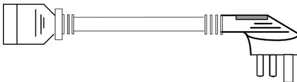
The AC power cable (ZJN.BH4.855.080-B) which meets German standard is composed of German standard French-mode two-plug connector and pins terminal, as shown in Figure 4-2.
