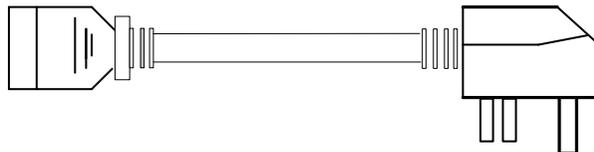
The AC power cable which meets North American standard (ZJN.BH4.855.035-G) is composed of North American standard three-plug connector and pins terminal, as shown in Figure 4-12.
