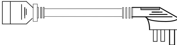
The AC power cable (ZJN.BH4.855.080-E) which meets Japanese/American standard is composed of Japanese/American standard two-plug connector and pins terminal, as shown in Figure 4-4.
